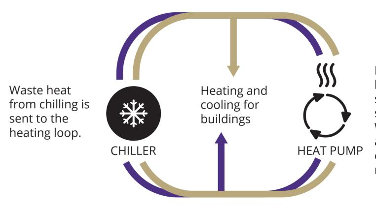
Heat pumps transfer heat from one source (such as a sewer line or Lake Washington) to another to either cool or heat as needed.
